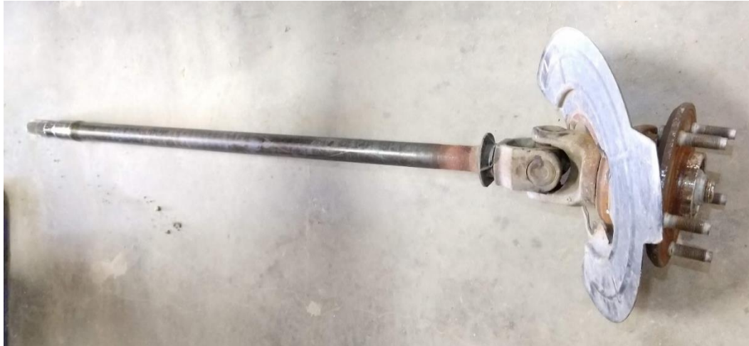
Figure 6. Passenger (Right) Side Axle and Unit Bearing Assembly
