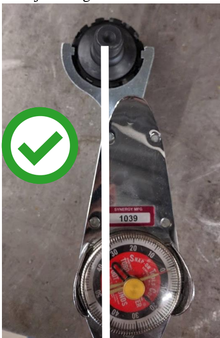
Figure 19. Correct Wrench Orientation
