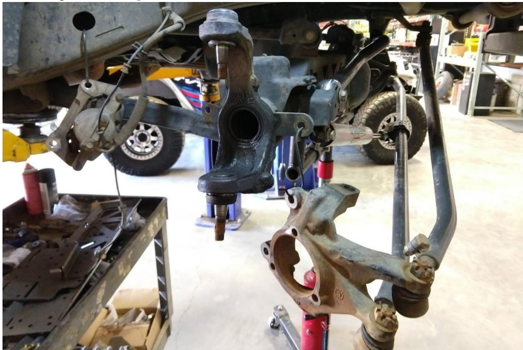
Figure 7. Knuckle Removed, Hanging from Axle Housing
