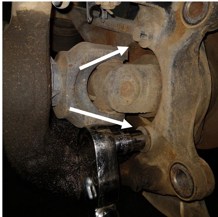
Figure 5. Unit Bearing/Hub Bolts on Back Side of Knuckle
