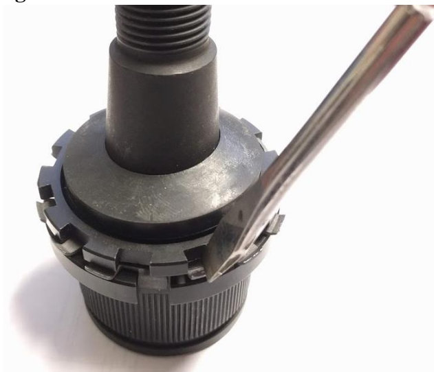
Figure 18. Bending Locking Tabs Back
