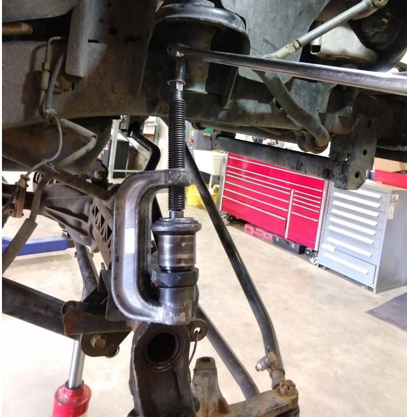
Figure 12. Pressing the Upper Ball Joint into Housing
