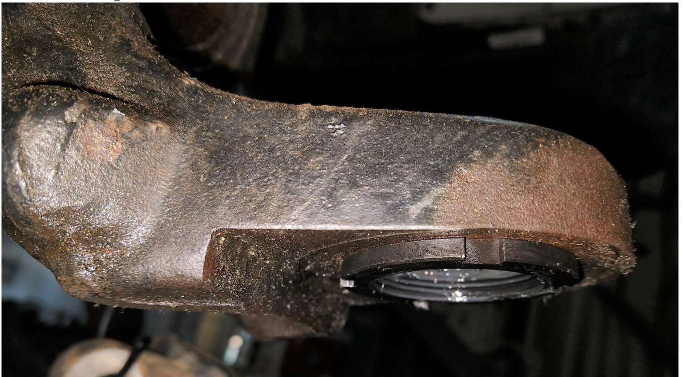
Figure 11. Lower Ball Joint Body Pressed In
