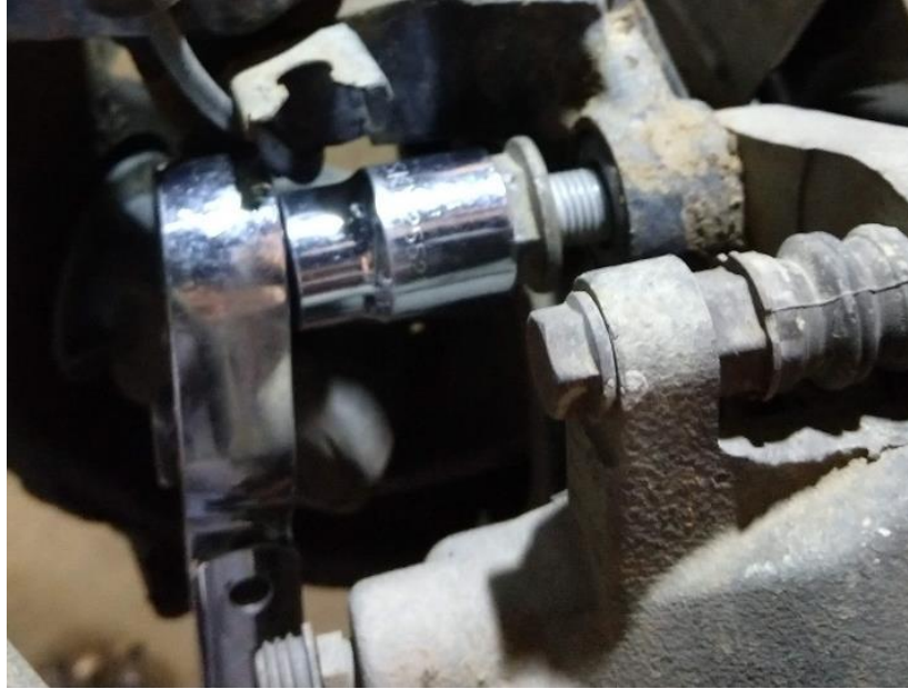
Figure 2. Removing Brake Caliper Carrier Bolts
